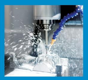
So-called multi-spindle machining centers combine several machining processes in one machine. During milling and drilling, a water-miscible cooling lubricant used at the individual machining stations is extracted directly at the machine and processed in a filter system.
